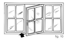
Doors and windows of room to be airconditioned are closed (with the exception of temporary installation where a partially opened window is necessary).
